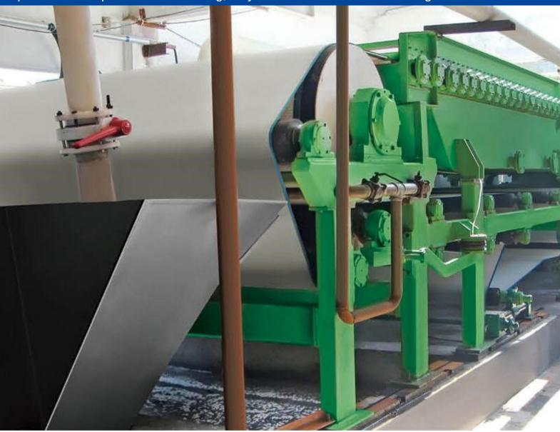
Pulp Washing Mesh Fabric for Belt Pulp Washer
